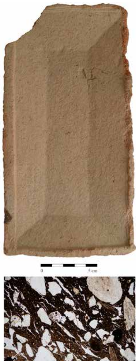
Fig. 13. Body fragment of a mirror tile, Petrov, Brno (photo V. Nosek), microstructure of the sample (photo M. Hložek), photomontage by Š. Trávníčková.
