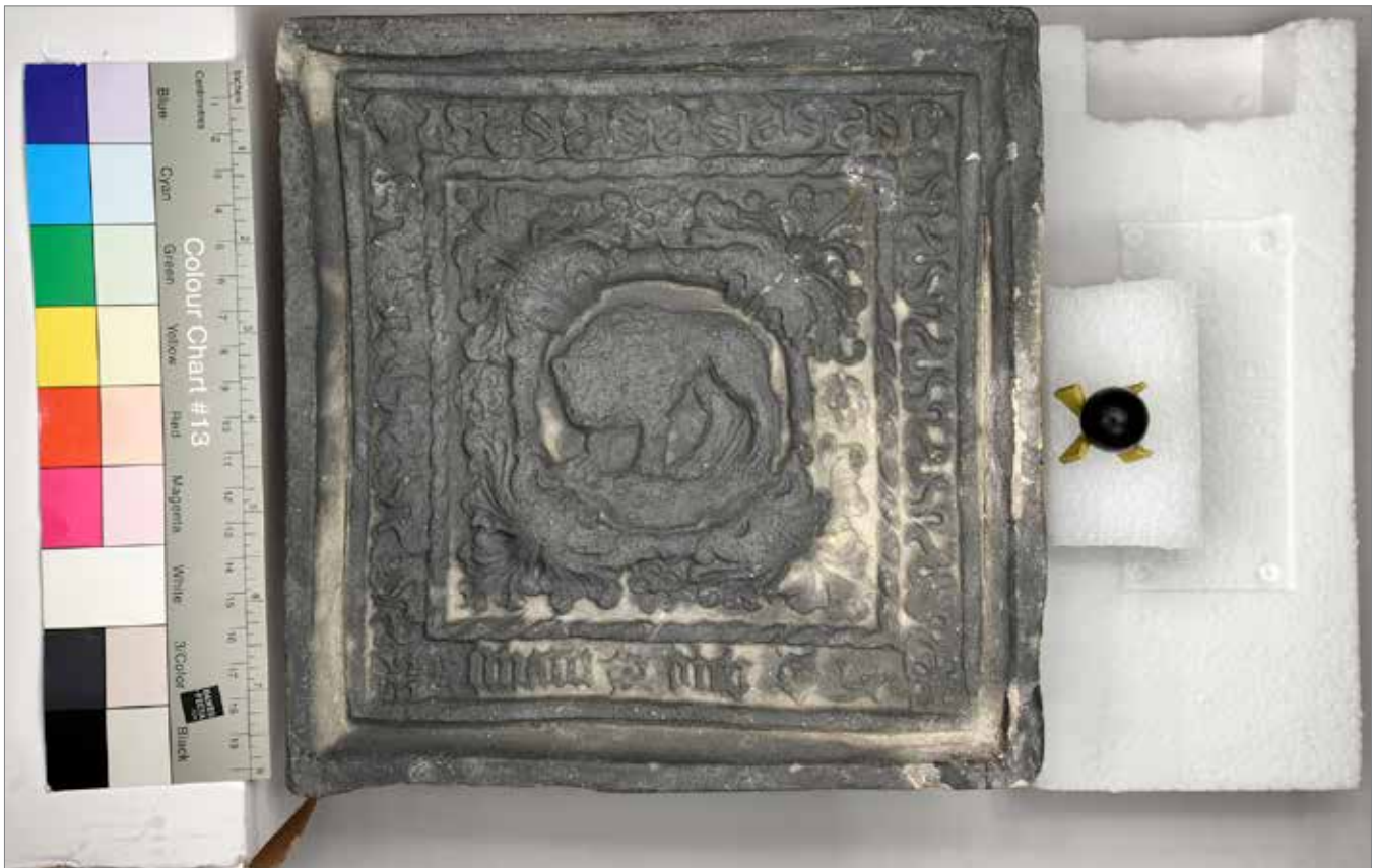
Fig. 9. Imaging area for the RTI method. Colour chart – artefact – reference marker.
