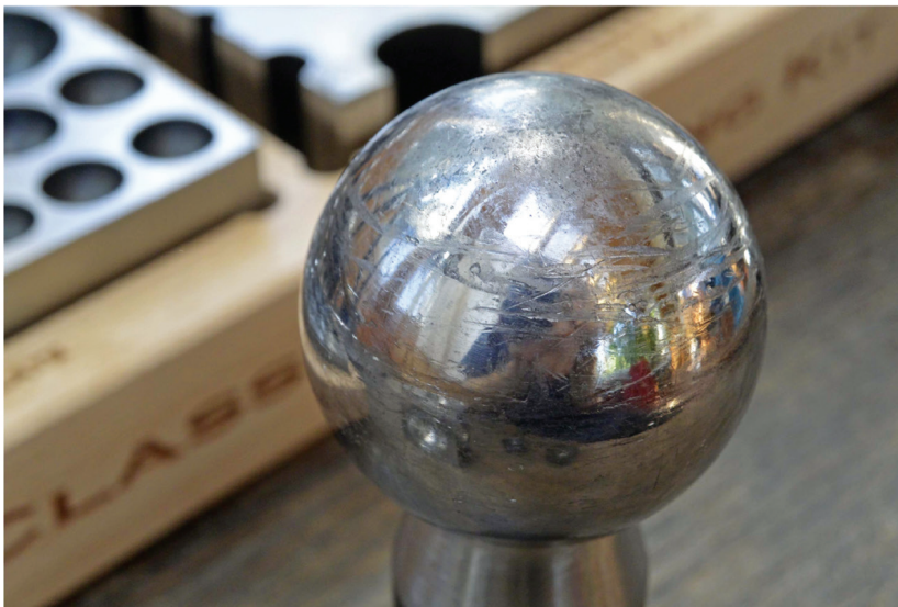
M - Deformed surface of spherical punch by cold forging sheet iron
