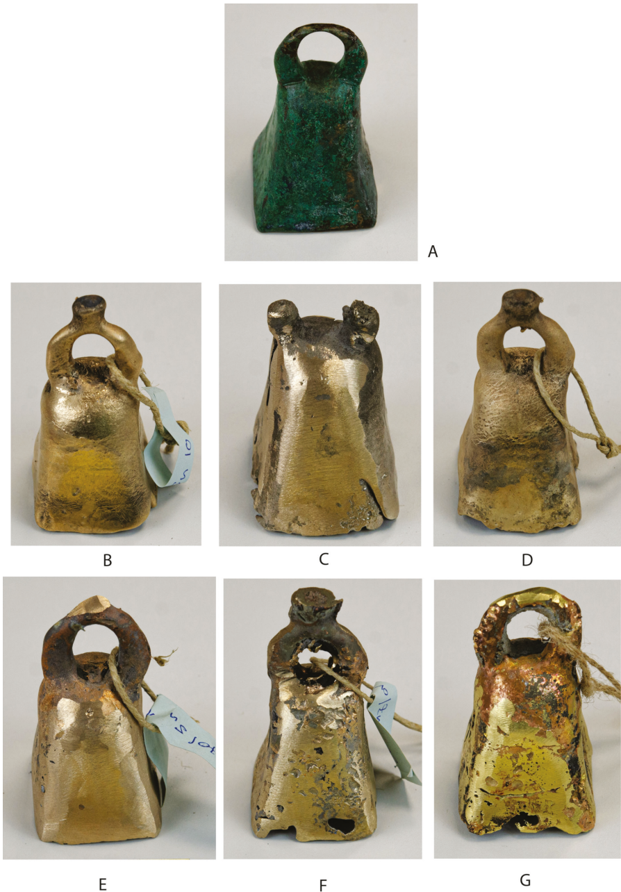
Fig. 7. The original Roman Bell Nr. 89 from Ovilava and its replicas. A – Roman bell Nr. 89, Ovilava/Wels, bronze; B – alloy I (bronze); C – alloy II (bell bronze); D – alloy III (leaded bronze); e – alloy IV (leaded bronze); F – alloy V (red bronze); G – alloy VI (brass). (Photos: J. Mühlhans, B. M. Pomberger)
