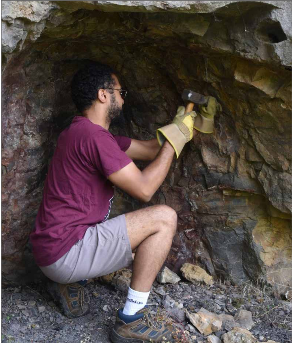
Figure 6. Removing the rock weakened by fire with tools.
